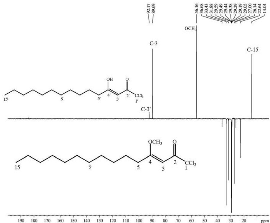
Figure S14. ^{13}\text{C} NMR DEPT135 spectrum (100 MHz, \text{CDCl}_3 ) of 1,1,1-trichloro-4-methoxy-3-pentadecen-2-one (91%) + 1,1,1-trichloropentadecan-2-one (9%).
