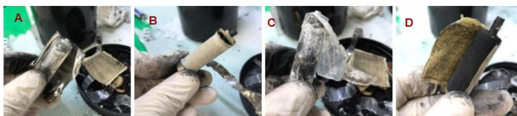
Figure S1. Disassembly sequence of the batteries to remove the graphite electrode.
