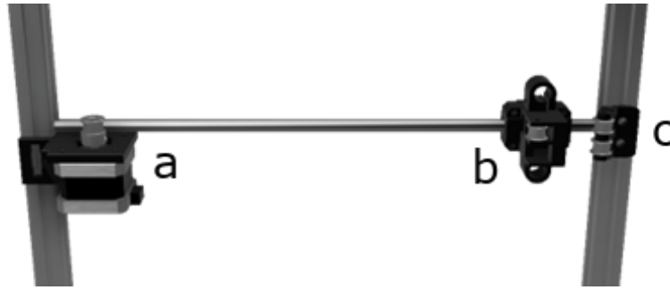
Figure S3. (a) Stepper motor with a pulley for a 6 mm GT2 belt, mounted to the aluminum profile using a PLA-printed part and secured with screws. (b) Carriage featuring a toothed tensioner pulley responsible for motion transmission. (c) PLA-printed part attached to the aluminum profile with smooth tensioning rollers to maintain belt tension. This system is mirrored on the opposite side of the machine.
