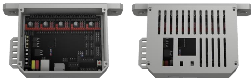
Figure S9. 3D-printed protective housing for the BTT SKR v1.4 motherboard.
