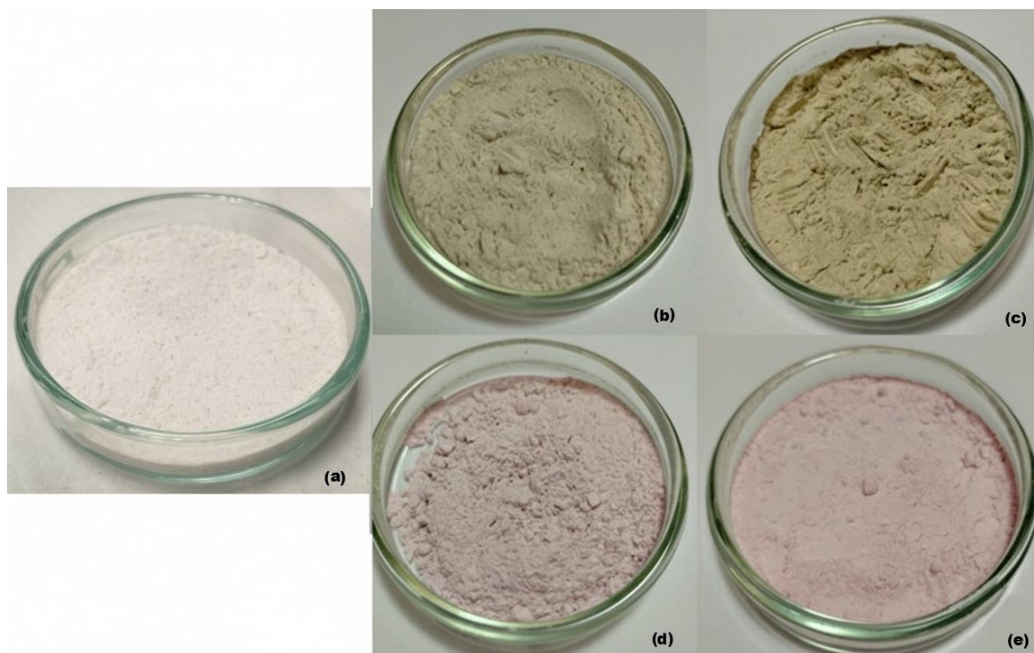
Figure S1. Optical comparison of the synthesized samples: (a) Si; (b) Si-Fe 5%; (c) Si-Fe 10%; (d) Si-Co 5%; (e) Si-Co 10%.
